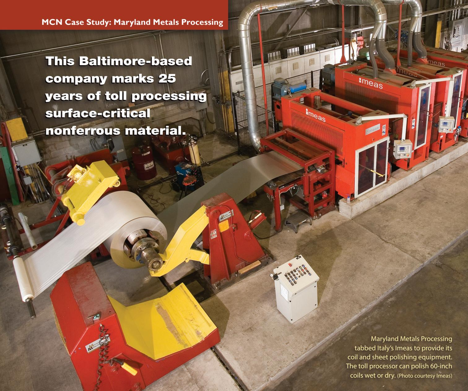
Maryland Metals Processing tabbed Italy's Imeas to provide its coil and sheet polishing equipment. The toll processor can polish 60-inch coils wet or dry. (Photo courtesy Imeas)
